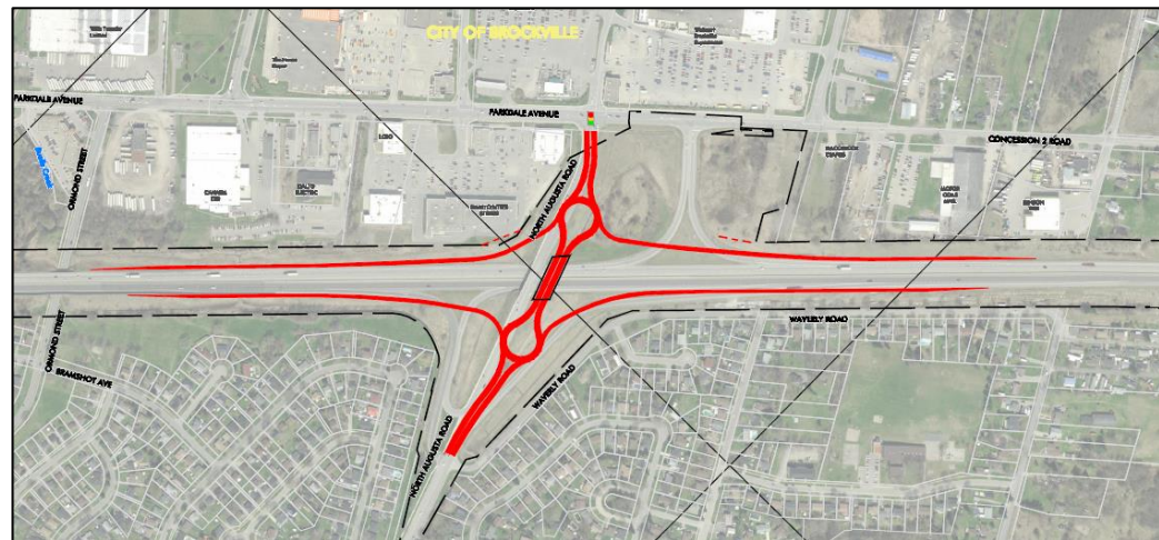
Figure 13: Alternative 3- Diamond with Roundabouts
